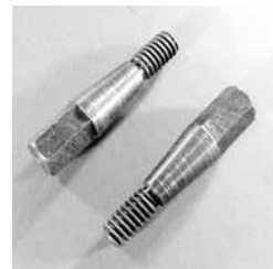
TC-88 Oil Pump Alignment Tool Tapered tool threads into the oil pump and perfectly aligns the pump to the cam plate. Use on all TC-88 engines. 5894
